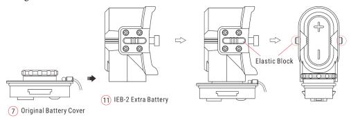
• To open the extra battery compartment cover, press the elastic blocks on both sides.
